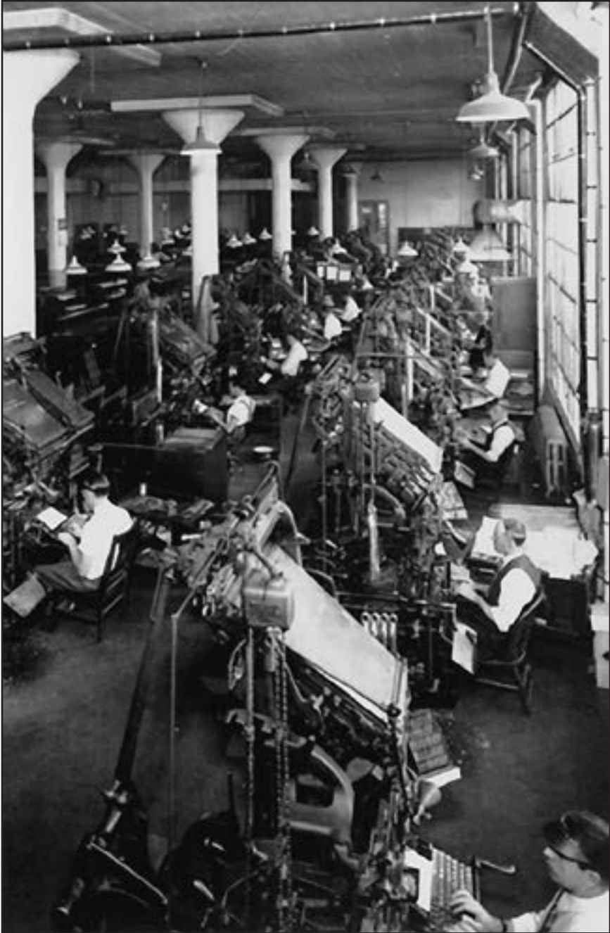
Linotype machines at the Office of State Printing, circa 1940. These machines have been replaced by computer publishing methods.
